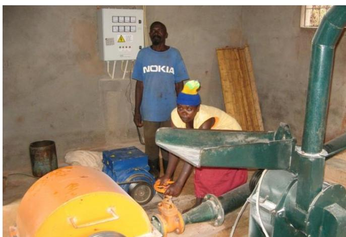
**Figure 3: Taking mechanical power off a micro hydro installation in Mozambique to drive a maize mill (credit: S. Trace)**
